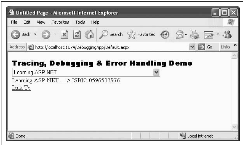
Figure 8-2. Here's DebuggingApp in action. After you select a book title from the DropDownList , its title and ISBN are output in the Label .
