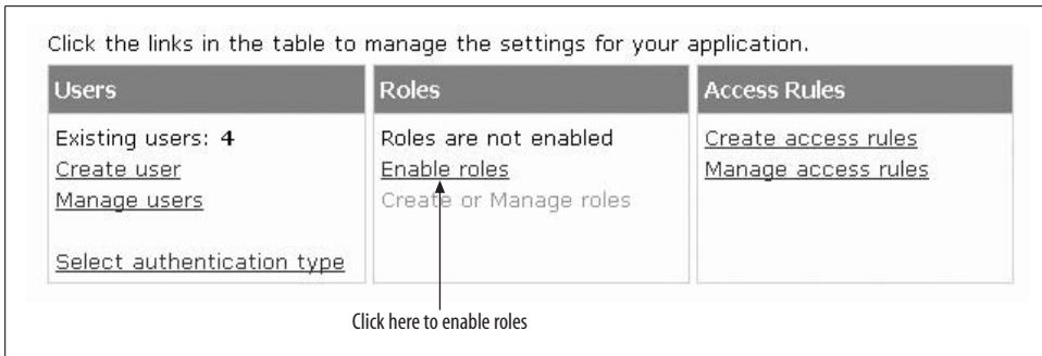
Figure 9-17. Click the Enable Roles link on the Security Page of the Web Site Administration Tool (WAT) to enable roles.
