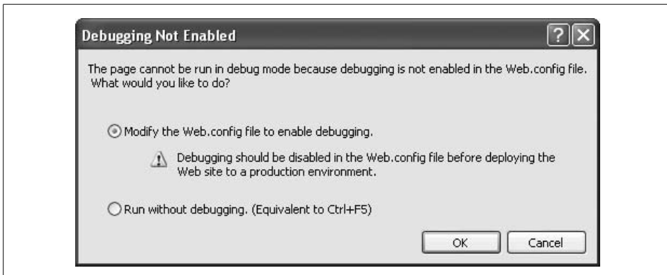
Figure 1-7. You'll see this Debugging Not Enabled dialog box the first time you run your application. Just select the first option and click OK to keep going.
